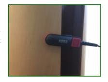
How to store the contact Microphone: always detach from the tuner and loosely wind the lead.
